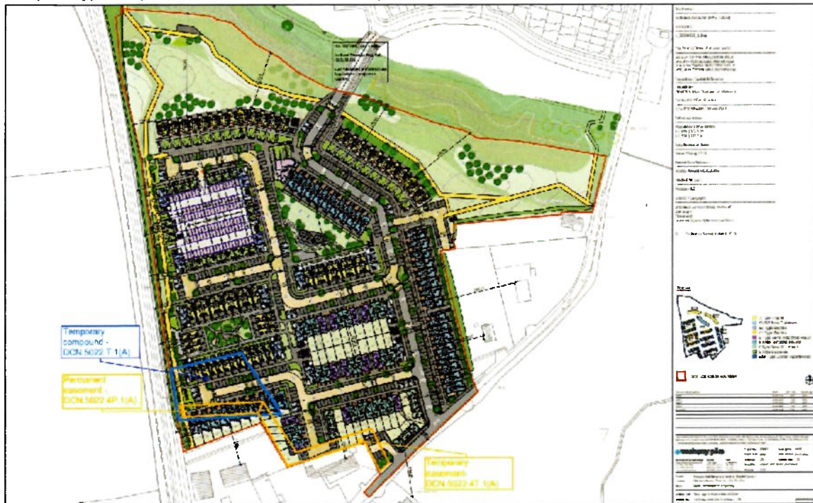
Figure 1: Indicative overlay of proposed temporary compound and easements (permanent & temporary) with permitted residential development site layout
