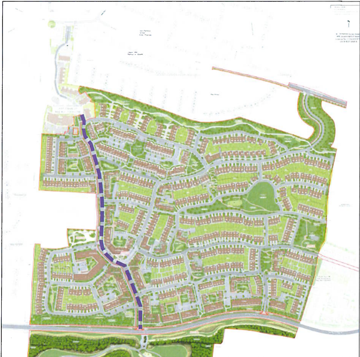
Figure 6: Permitted Haul Route – Suitable Location for Temporary Right of Way in the event the Railway Order is Implemented in Advance of Phase 1 and/or LRD Permission
